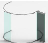
Panels can move through angled openings and several corners, stacking to one or both ends.
